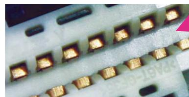
The metal terminal to grip the terminals of the ECU is properly opening. (see photo)
