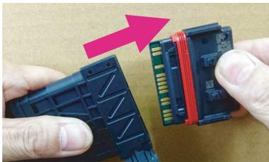
② When you pull the lever all the way, the ECU will become free. Grasp the coupler body firmly, pull the ECU straight out. Do not touch the terminals of the ECU with your hands.
