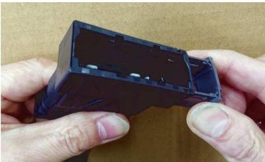
① Check that there is no dust or debris in the coupler slot of the product. Next, make sure that the gray lever is pulled all the way out.
