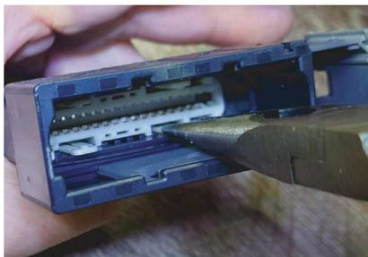
Using radio pliers or similar tools, pull horizontally and gradually so as not to damage the wide claws that protrude from four locations on the top, bottom, left, and right sides of the white part at the back inside the coupler slot. Once the terminal looks like the "correct example", do not pull it any further.
