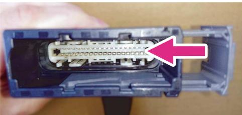
② **Every time** make sure that the metal terminal inside the coupler slot (see photo) is open. Make sure that the metal terminals on the arrow part open evenly and that there is a gap for the "plug-in part" of the ECU to enter. Do the same for the body side coupler.
