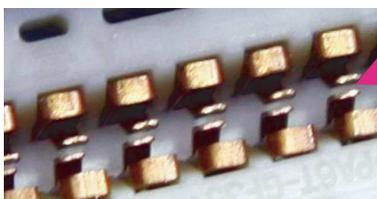
The metal terminal to grip the terminals of the ECU is popping out. (see photo)
