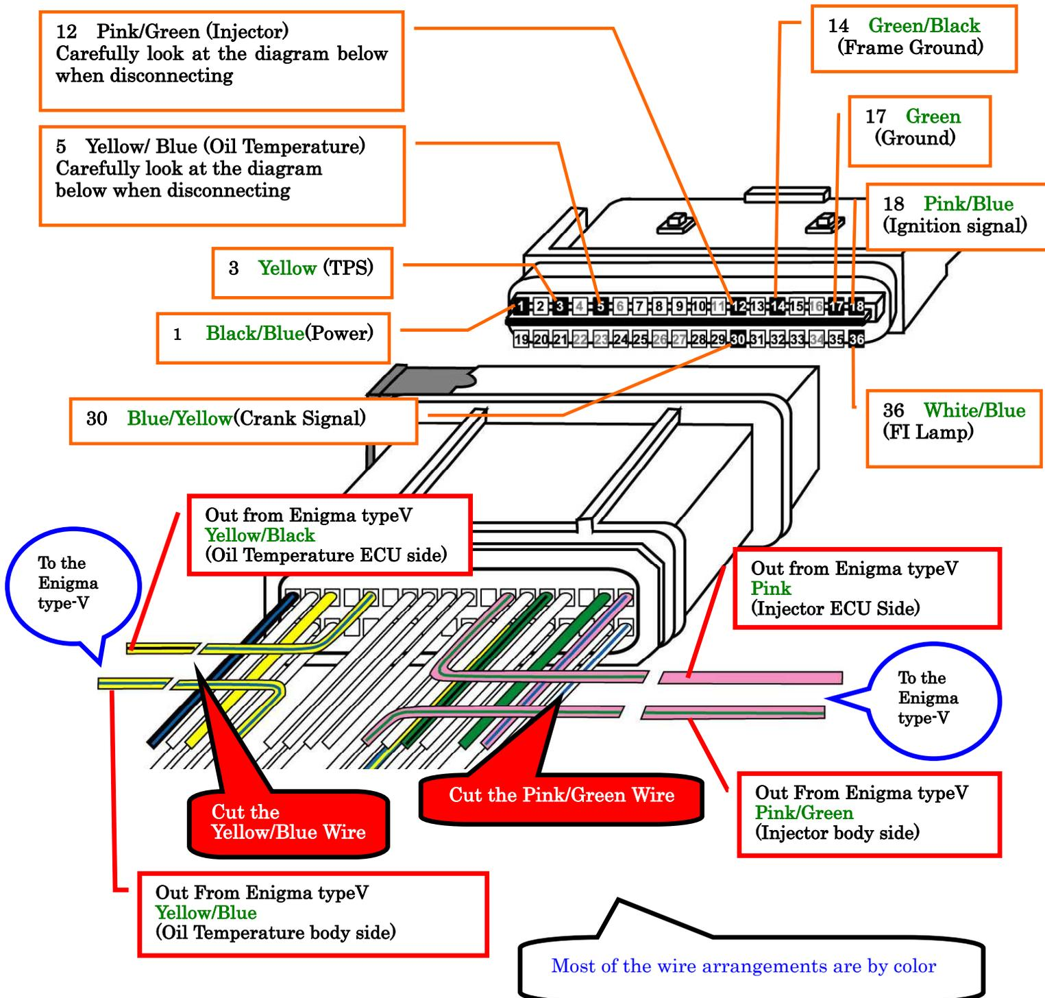
ECU terminal connected 9wires 1, 3, 5, 12, 14, 17, 18, 30, 36. Please confirm the picture.
