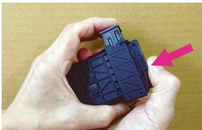
① Check the orientation of the ECU, insert it slowly. If you mistake on the front and back, can not insert the coupler slot. Push the ECU body straight into the coupler.
