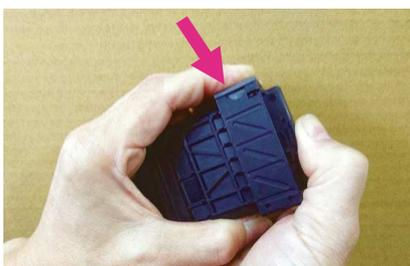
② While pushing the ECU, push the gray lever back to its original position. At this time, the ECU is linked to the movement of the gray lever. The system goes deeper and is set in the correct position.
