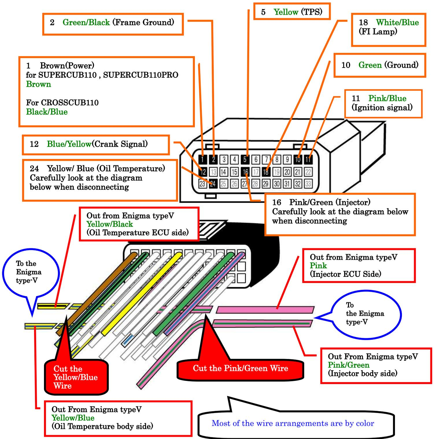
ECU terminal connected 9wires 1,2,5,10,11,12,16,18,24.Please confirm the picture.
