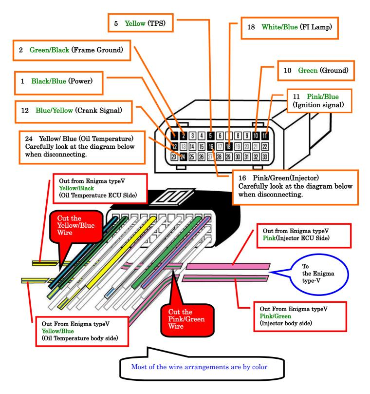
ECU terminal connected 9wires 1,2,5,10,11,12,16,18,24.Please confirm the picture.
