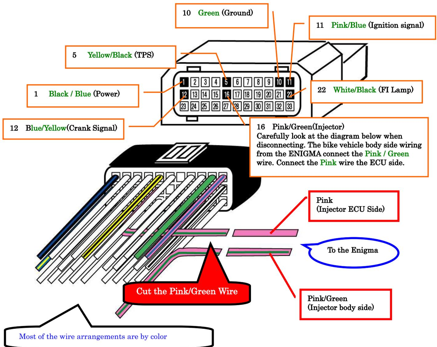
ECU terminal connected 7wires 1, 5, 10, 11, 12, 16, 22. Please confirm the picture.
