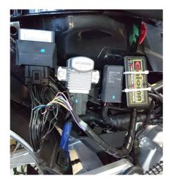
Remove the coupler connected to the ECU, process the wiring and interrupt ENIGMA. Install ENIGMA close to water.
