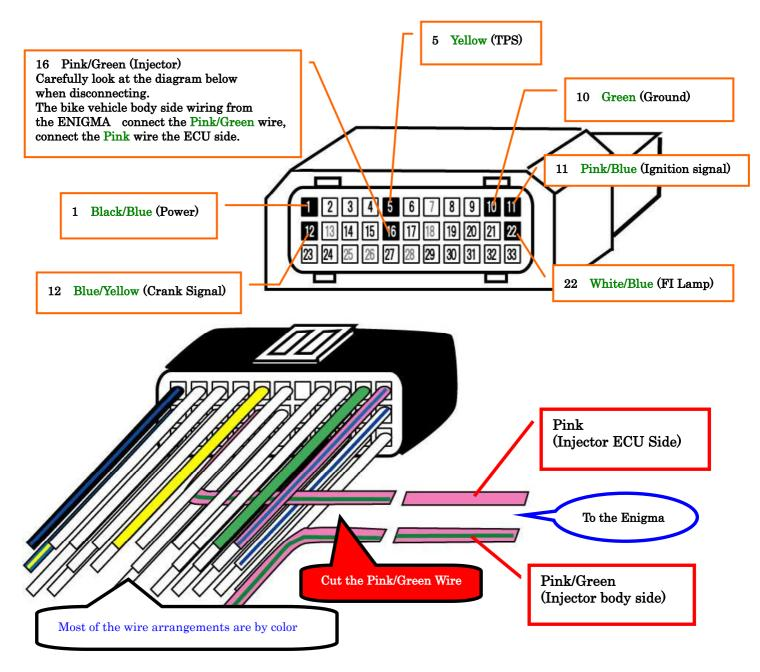
ECU terminal connected 7wires 1,5,10,11,12,16,22. Please confirm the picture.
