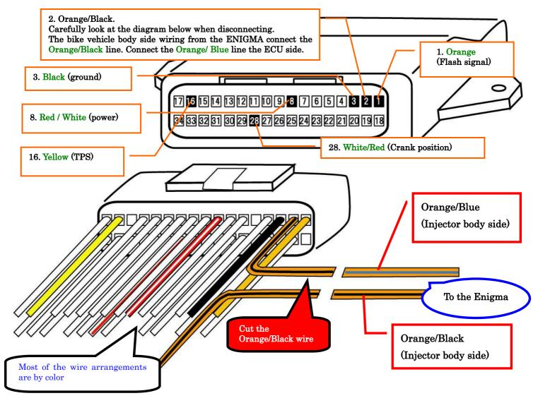
ECU terminal connected 6wires 1,2,3,8,16, 28. Please confirm the picture.
