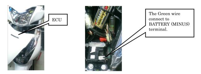
Installation should be done in a safe place. A basic knowledge of <u>LEAD125</u> maintenance is necessary. There is an ECU back around the lower right frame under the right front tire slightly and remove the exterior around the lid of the gasoline cock of feet ahead of the normal vehicle is attached. Remove the 33pin coupler then the ECU.
