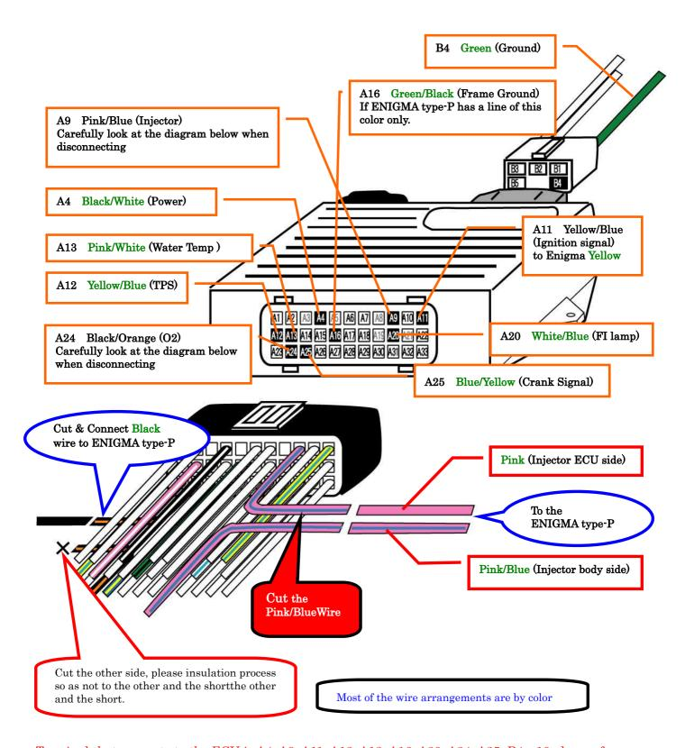
Terminal that connects to the ECU is A4, A9, A11, A12, A13, A16, A20, A24, A25, B4 10 places of. Please check the above diagram.
