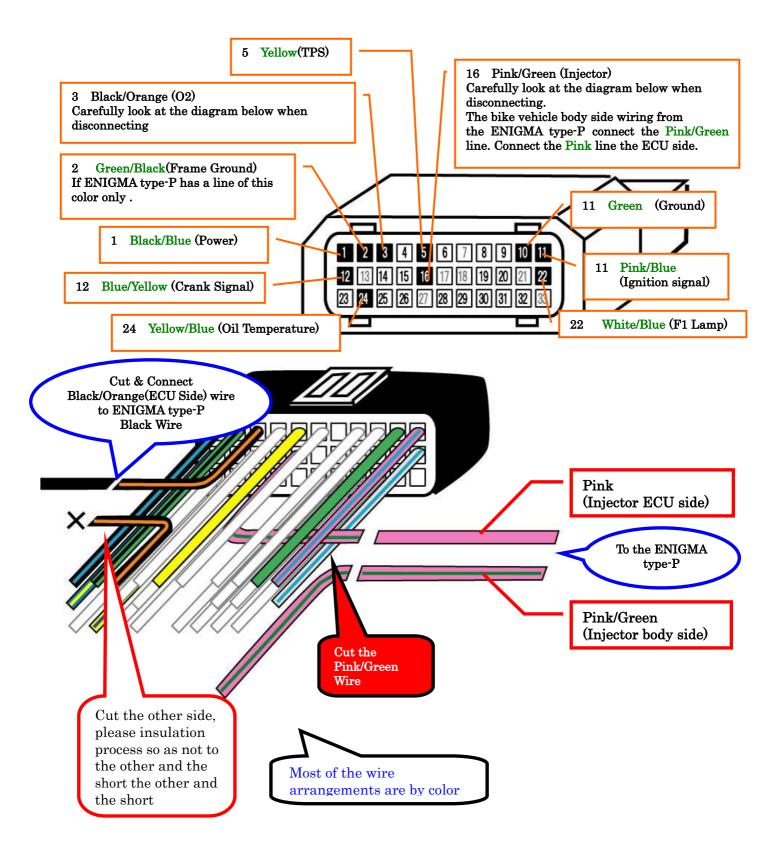
ECU terminal connected 10wires 1, 3, 5, 10, 11, 12, 16, 22, 24. Please confirm the picture.
