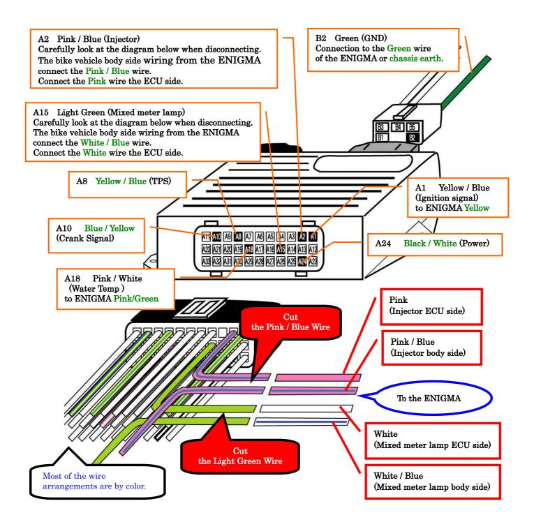
Terminal that connects to the ECU is A1, A2, A8, A10, A15, A18, A24, B2 8 places of. Please check the above diagram.
