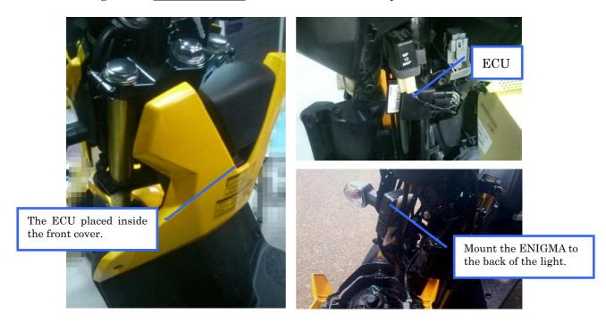
On a standard bike, the ECU placed inside the front cover. The ECU is rubber-mounted when the front cover is removed. Mount the ENIGMA to the back of the light.
