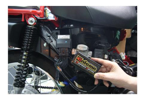
If you use the RTF type, remove the coupler which is connected to the ECU, please connect the coupler that has come out from ENIGMA LC RTF to the ECU and the vehicle body side. Please make sure that the lock sound is a "click".
