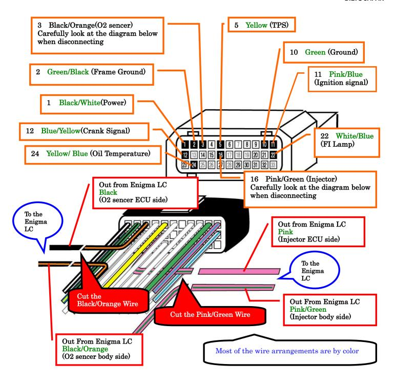
ECU terminal connected 10wires 1,2,3,5,10,11,12,16,22,24. Please confirm the picture.
