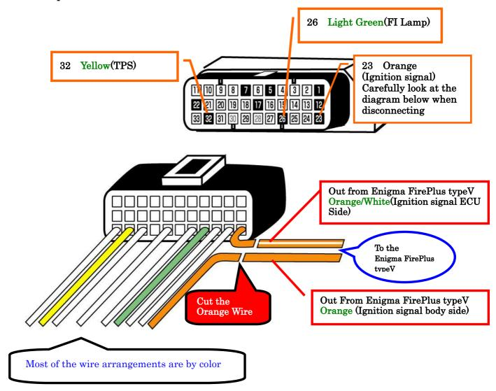
ECU terminal connected 9wires 1, 5,7,12,17,22,23,26,32. Please confirm the picture.
