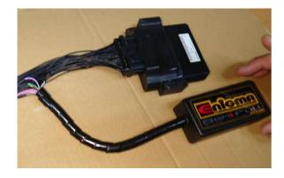
Disconnect the ECU from the body coupler and connect the ENIGMA coupler between the ECU and the body coupler. Attach the ECU to the ENIGMA coupler.
