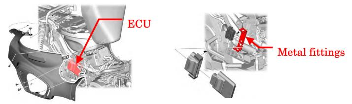
Remove the center cover -> the legshield -> the main pipe cover -> the side cover -> the body cover in accordance with the service manual.
