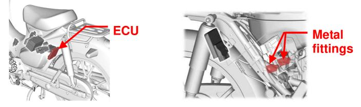
Remove the rear fender -> the rear inner fender in accordance with the service manual. The ECU is secured by a rubber cover that is inserted into a metal fitting protruding from the main unit. Remove the ECU with the rubber cover by pulling the rubber cover.
