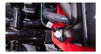
Place the ECU and the ENIGMA between the the rear fender to the rear inner fender. The ENIGMA body must be secured against excessive vibration and rainwater. Connect the wires with Y-terminal terminal that branches out from the middle of the ENIGMA RTF to the frame using the screws or similar securing under the rear center cover.
