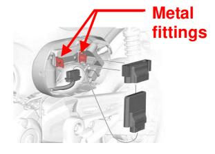
Remove the outer side cover in accordance with the service manual.
