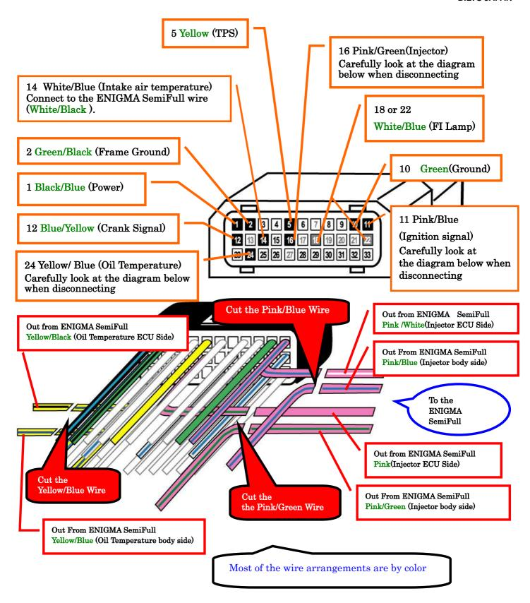
ECU terminal connected 10wires 1, 2, 5, 10, 11, 12, 14, 16, 18 or 22, 24. Please confirm the picture.
