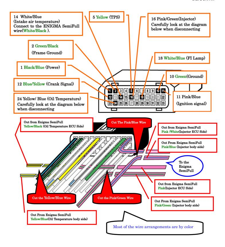
ECU terminal connected 10wires 1, 2, 5, 10, 11, 12, 14, 16, 18, 24. Please confirm the picture.
