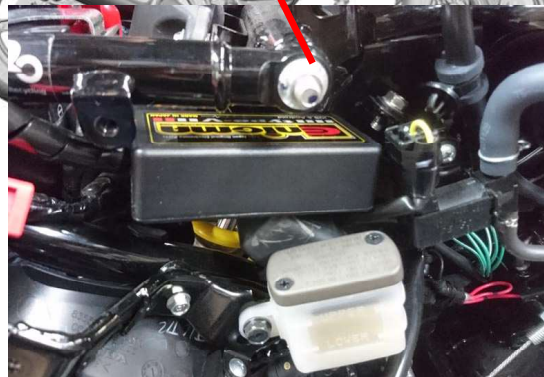
Example of ENIGMA mounted inside the right side cowl
