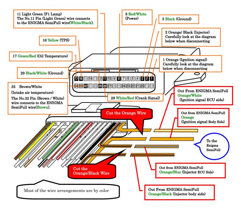
ECU terminal connected 10wires 1,2,3,8,11,16,17,28,29,32. Please confirm the picture.
