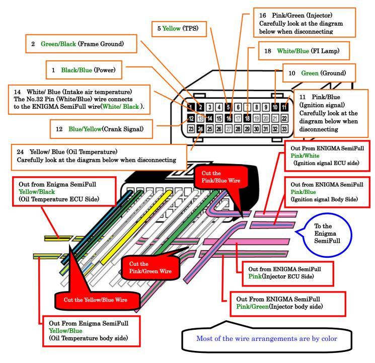
ECU terminal connected 10wires 1,2,5,10,11,12,14,16,18,24. Please confirm the picture.
